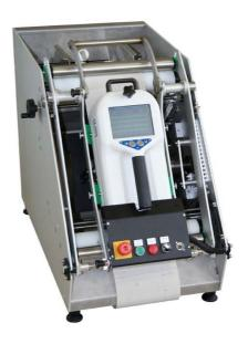
By means of a calibration check plate, the proper function and calibration of the FX 3360 PORTAIR can be checked in a matter of seconds.
