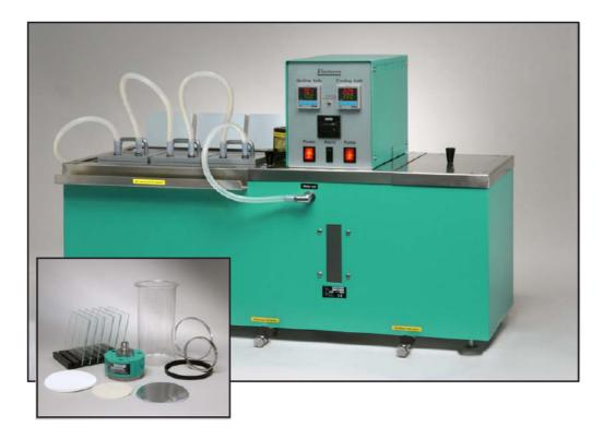
Equipment for determination of windscreen fogging according to ISO, DIN, ASTM and other automotive standards. The equipment has a compact design with the heating bath and cooling bath integrated in one casing. For cooling the water bath, the instrument is normally connected to tap water of max 18 °C. If the tap water is too warm, a model EB 03C can be supplied with a built in cooling system with Peltier elements.
