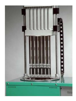
**TR Tester, ET 01,** for determination of low temperature characteristics by the temperature retraction procedure according to ISO 2921 and ASTM D-1329.
