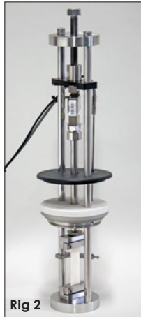
Rig 2 is arranged for testing in tension according to ISO 6914 method A.
