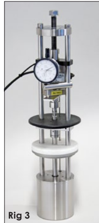
Rig 3 is arranged for testing in liquid according to ISO 3384.
