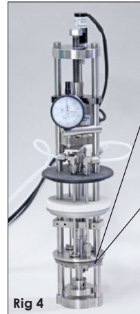
Rig 4 is arranged for testing according to ALE-test.
