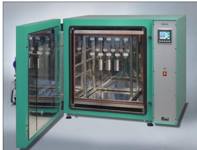
The Film Creep Tester has a fixed set air exchange rate, 7 or 14 changes per hour. It includes hooks to hang 10 test pieces 25 × 100 mm and 10 sets of grips to attach to the test pieces, together with weights, 1,3 kg and 2,3 kg.
