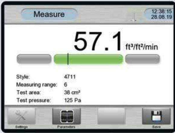
Touch display for operation of the instrument
